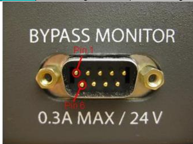
Figure 7: DB9 Pinouts for Remote Bypass Control
