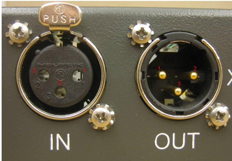
Figure 4: XLR Connection Pinouts
