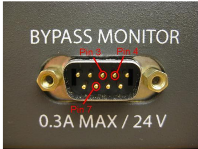
Figure 6: DB9 Pinouts for Remote Bypass Monitoring
